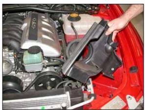
10. Lift up and pull out the air deflector from behind
