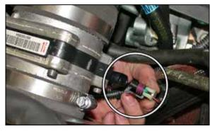
30. Reconnect the mass air sensor electrical connection.
