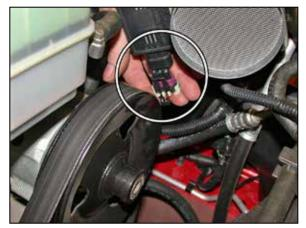
6. Release the mass air sensor electrical connection clip, then disconnect the electrical connection.
