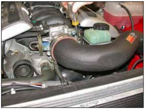
17. Install the K&N<sup>®</sup> intake tube onto the throttle body as shown and secure with the provided hose clamp, using the 8mm bolt provided. Secure the K&N<sup>®</sup> intake tube onto the mounting bracket installed in step #12.
