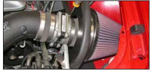
29. Install the air filter assembly onto the K&N<sup>®</sup> intake tube and secure with the provided hose clamp.
