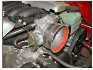
13. Install the silicone (08755) onto the throttle body and secure with the provided hose clamp.
