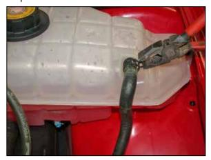
21. Using a pair of pliers, loosen the spring clamp on the coolant reservoir hose. rotate the coolant hose 90 degrees down as shown. Then resecure with the stock clamp.
