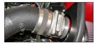
28. Install the mass air sensor assembly onto the  $K\&N^{\odot}$  intake tube and secure with the provided hose clamp.
