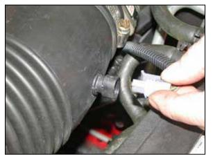
4. Release the air temp. electrical connection clip, then disconnect the electrical connection.
