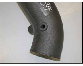
15. Install the provided rubber grommet into the  $K\&N^{\ensuremath{\$}}$  intake tube as shown.
