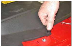
33. Reinstall the five radiator cover retaining clips removed in step #2.
