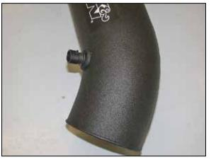
16. Install the air temperature sensor from step #14 into the grommet in the K&N<sup>®</sup> intake tube as shown.
