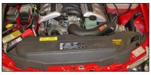
32. Reinstall the radiator cover removed in step #3.
