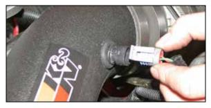
31. Reconnect the temperature sensor electrical connection.
